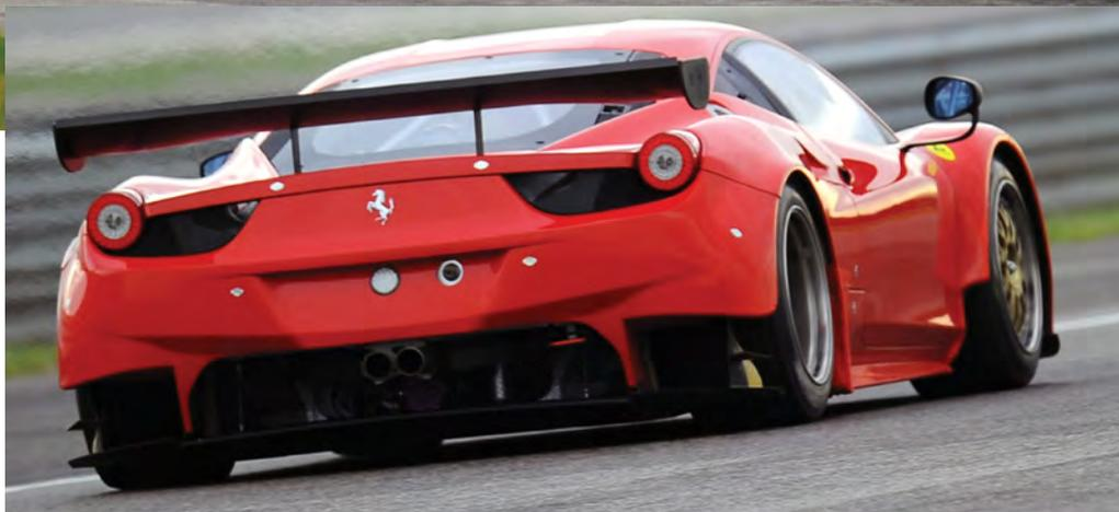
**At the rear, the bumper has been redesigned to improve the extraction of the air and to make the diffuser more efficient. The wing now has a different profile and features the mandatory 25mm Gurney flap**
