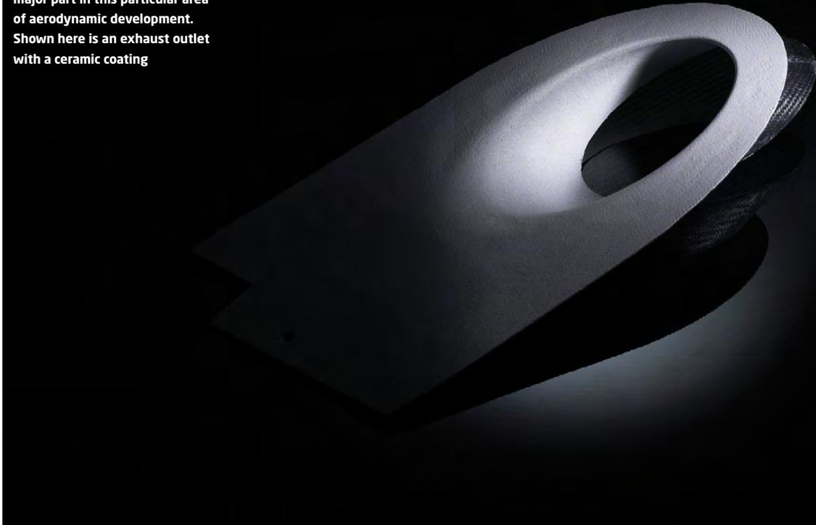
very strange things. The radius and the contact patch changes continuously, and this is a very important aspect in terms of aerodynamics, especially in open-wheel cars. At the base of the tyre there is a vortex created and, if this gets into the diffuser, it reduces its effectiveness. Using the mass flow from the exhaust to drive this vortex away from the diffuser and other critical areas effectively makes the diffuser larger and more efficient.'
