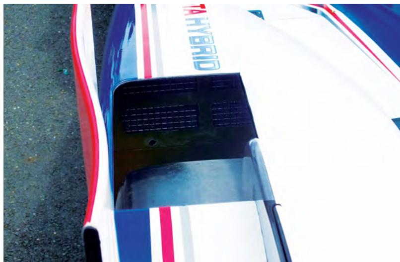
The TS030 features cooling holes on the inner face of the rear wheel arch, one of the few locations where openings are allowed under the car
