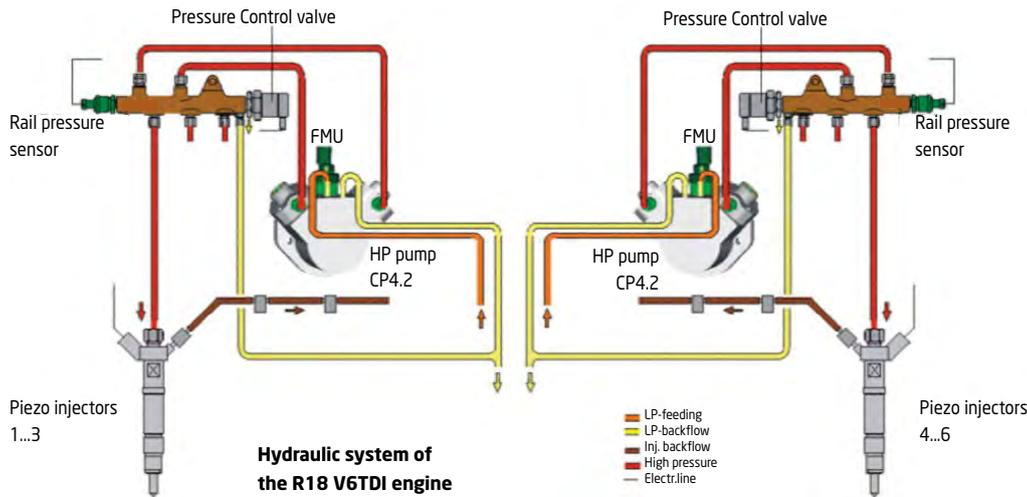
**The hydraulic system of the R18 V6 TDI engine**
