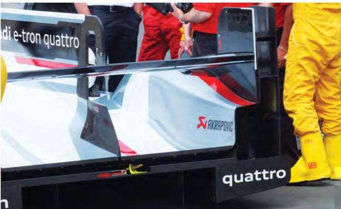
The Audi's Le Mans specification rear end features a lower rear wing. The double rear wing end plates are directly inspired by the TS030
