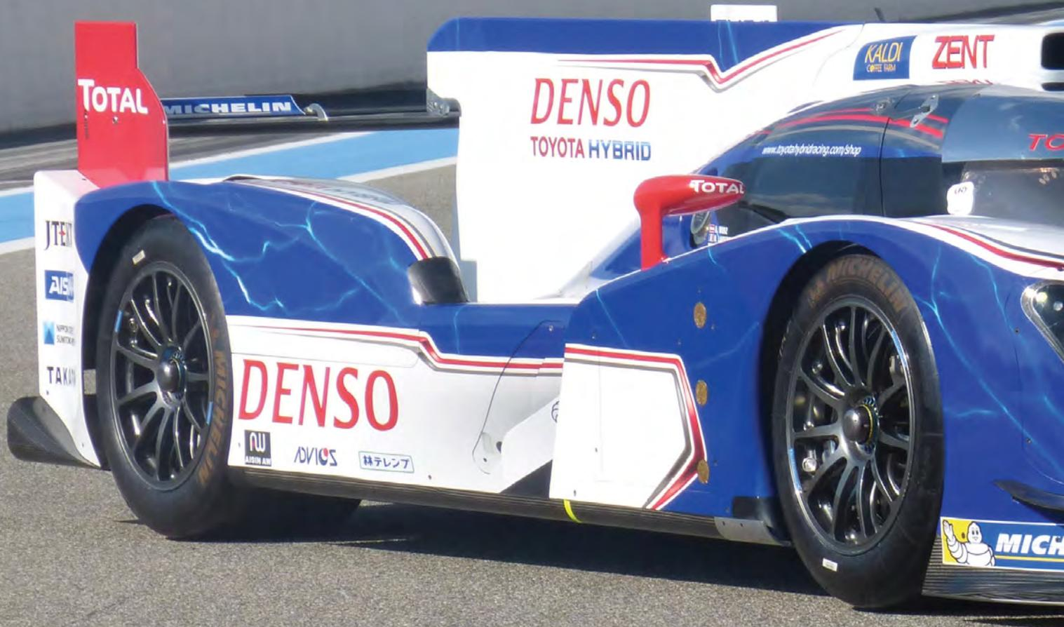
**T**oyota's 2013 Le Mans car is so similar to the 2012 machine that there is no new model designation, despite a new tub, a more central seating position for the driver to improve visibility, and a new aero package that is aimed at reducing the sensitivity of the car to changing conditions.
