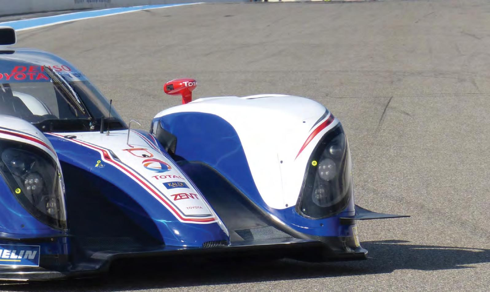
of 2012. The tub used last year was designed to evaluate both front and rear hybrid systems, and the team raced with the compromised chassis. Now that it has settled on a rear-only solution, the tub has changed to reflect that, leading to a new, tightly controlled aero package. The new nose is lower, and the change means that the team will have to re-crash test the tub ahead of its first race.
